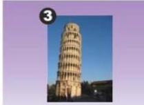
3 This tower is in Italy. It is actually a bell tower for the cathedral. The height of the tower is 55.86m on the low side and 56.7m on the high side. The tower has sunk on one side due to unsuitable foundations.
